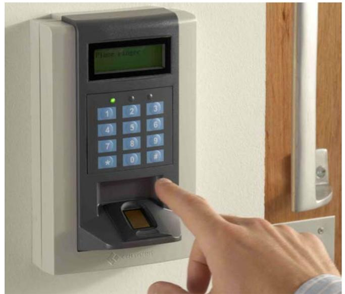
Featuring a controller, card reader and fingerprint solution in one device, the S610f is a fully integrated biometric and access control reader that is used as part of the AC2000 system. Fingerprint templates are captured on the AC2000 enrolment station at the same time as a cardholder's personnel details and images are captured and are then saved to the AC2000 server.
