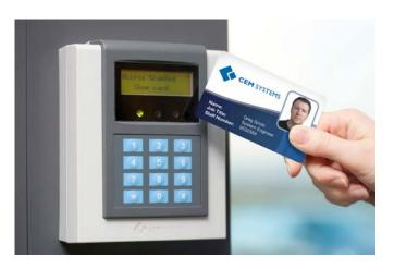
Over the years, the system at Steria has migrated from using legacy S600 readers to the current model – CEM's S610e reader. The S610e is an intelligent IP card reader which offers integral reading technology
